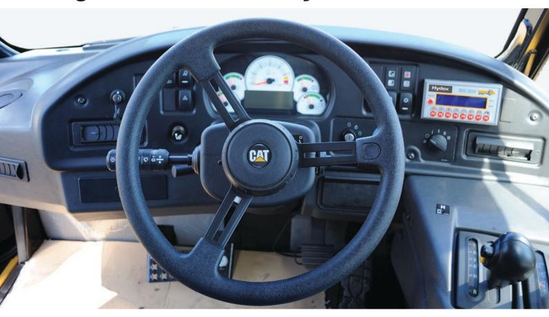
Available for all CAT® Articulated Dump Trucks, Hydex offers an optional weight measurement system. The system monitors the loading cycle in real time, so machine capacity can be fully utilised, while avoiding the dangers of overloading.
